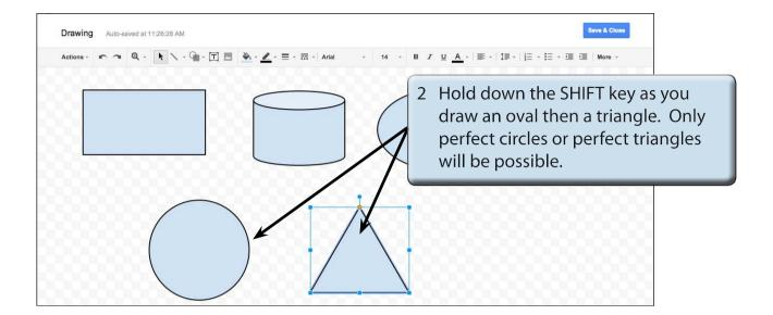
NOTE: i The SHIFT key causes all sides of an object to be the same size.
