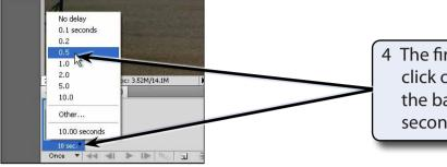
4 The first frame should be visible, click on the TIME DELAY value at the base of the frame and select 0.5 seconds.
