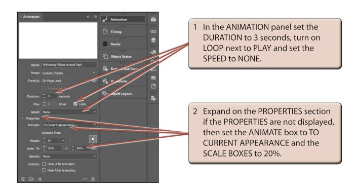
NOTE: These changes will cause the heading to start at 20% of its size, grow to its actual size then loop continuously.
