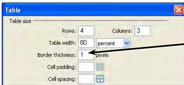
5 Set the BORDER THICKNESS box to 1 so that a thin line border will be inserted.
