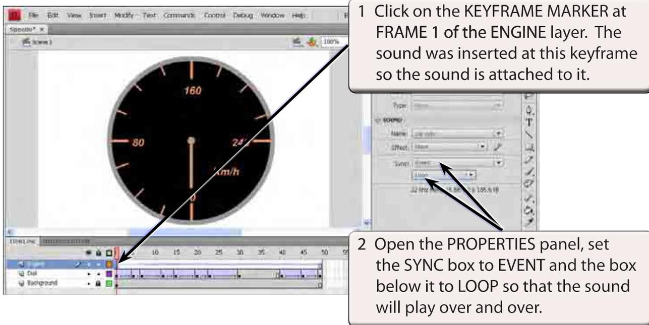
1 Click on the KEYFRAME MARKER at FRAME 1 of the ENGINE layer. The sound was inserted at this keyframe so the sound is attached to it.
