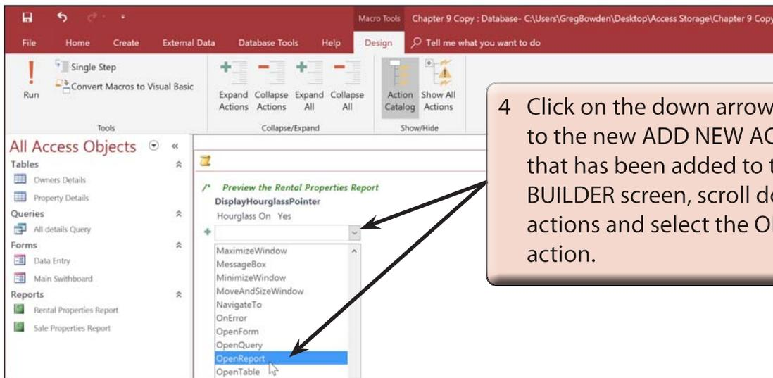
4 Click on the down arrow key next to the new ADD NEW ACTION box that has been added to the MACRO BUILDER screen, scroll down the actions and select the OPENREPORT action.
